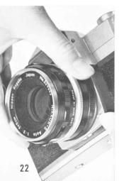
To remove the lens, hold the camera as shown left, depress the lock button found underneath the lens and turn the lens barrel clockwise until the black dot on the aperture indicator of the milled ring of the lens lines up with the black dot on the camera body.
