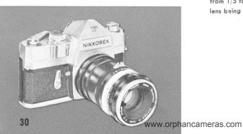
The extension tubes are fitted between a Nikkor F-mount lens and the Nikkorex camera body for taking close ups. One set consists of five tubes: A, B1, B2, C and D. The range of reproduction ratios obtained by selection and fitting together of the tubes is from 1/4.4 to 1/1 with 50mm and from 1/5 to 1/1.1 with 58mm focal length master lens being fully extended.
