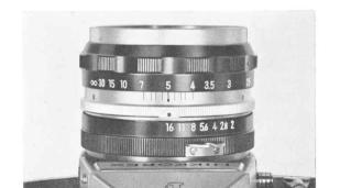
F: 16 opening (F: 16 is shown in blue), the depth of field indicated by the blue colored lines on either side of the black indicator line will be between 7 ft. or 2 meters and 4 ft. or 1.2 meters approximately. This means that a picture taken at F: 16 with the lens focused at 5 ft. or 1.5 meters will show a range of acceptable sharpness between 7 ft. or 2 meters and 4 ft. or 1.2 meters. The sharpest focus will be at 5 ft. or 1.5 meter.
