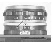
When taking infra-red pictures the distance setting obtained by focusing on the screen has to be adjusted before shooting. This is done by rotating the lens slightly, until the focused point on the distance scale is changed to align with the red dot on the depth of field scale.
